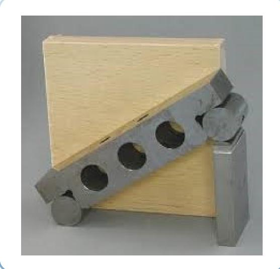
Slip gauges were first developed by Johnson, and sometimes also called as 'Johnson Gauge Blocks'. These are rectangular blocks of steel having a cross-section of about 32 mm x 9 mm.
