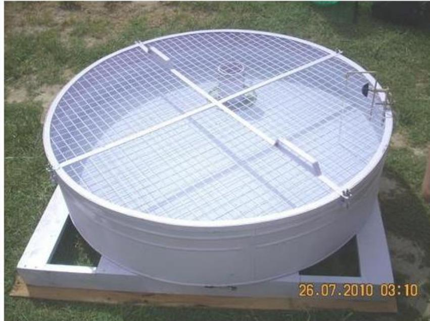
Fig. 25.3. Pan evaporimeter.
