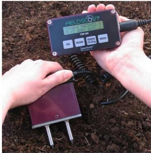
Fig. 24.5. TDR probe for soil water measurement.
