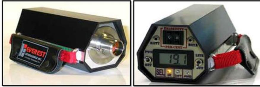
Fig. 27.5. Infrared thermometer for scheduling irrigations to crops.
