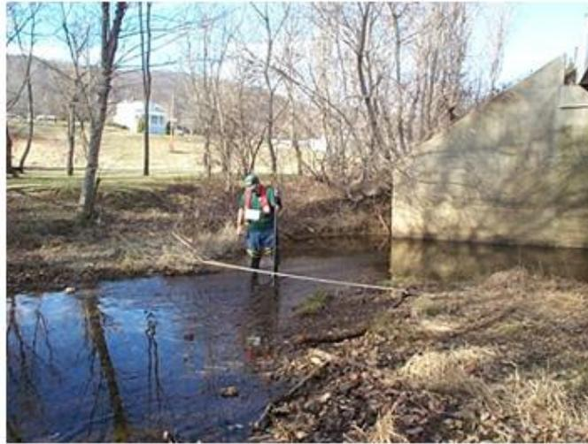
**Fig.5.3. Discharge measurement at a section.**
