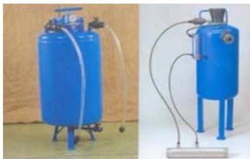
Fig. 43.2. By- pass pressure tank. (Source: Tiwari, 2009, pp. 591)
