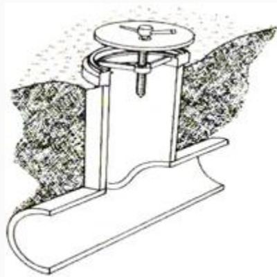
Fig. 15.5. Section of an alfalfa valve for a low head pipeline.
