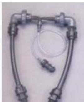
Fig. 43.3. Venturi Injector.
