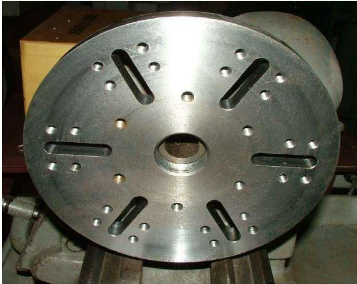
Face Plate fixed on the lathe chuck
