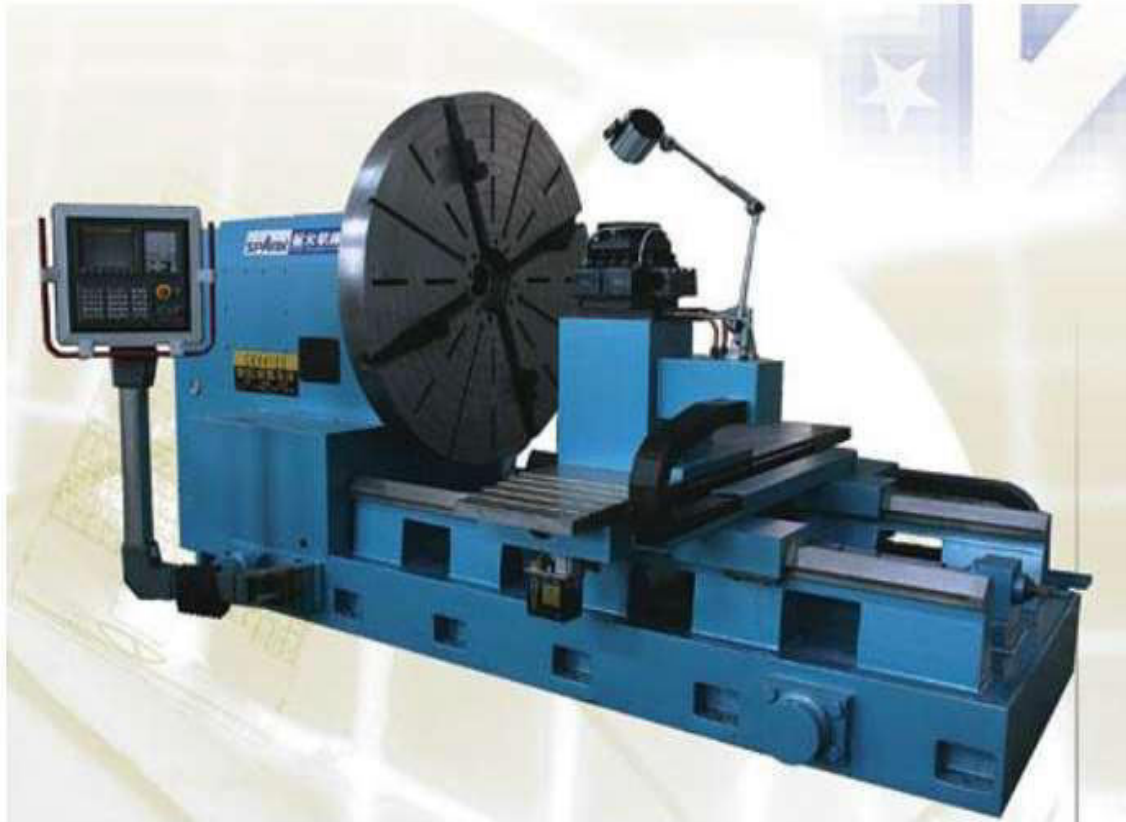
Face Plate fixed on the lathe chuck
